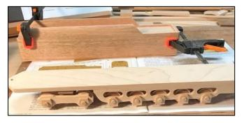
In fifteen days or so the 4-6-4 carriage was done. That's railroader-speak for 4 wheels in the front, 6 drivers in the middle and 4 wheels under the firebox and cab.
